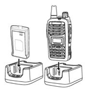
Plug the uncharged battery or transceiver with battery into charger, and make sure the battery contact with charging terminal. Red light means charging on, while green light means off.
